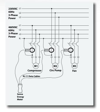
A true three channel meter allowing for measurement of various ampacities and voltages can reduce installation costs dramatically. Additionally, scaling the BACnet analog variable to "3" will scale the output for a balanced motor load.
